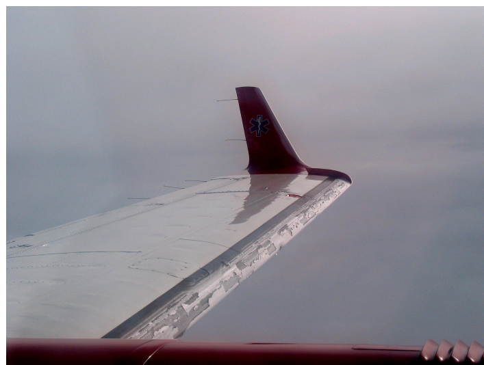
Figure 1. Ice accretion on the wing's leading edge [15].
