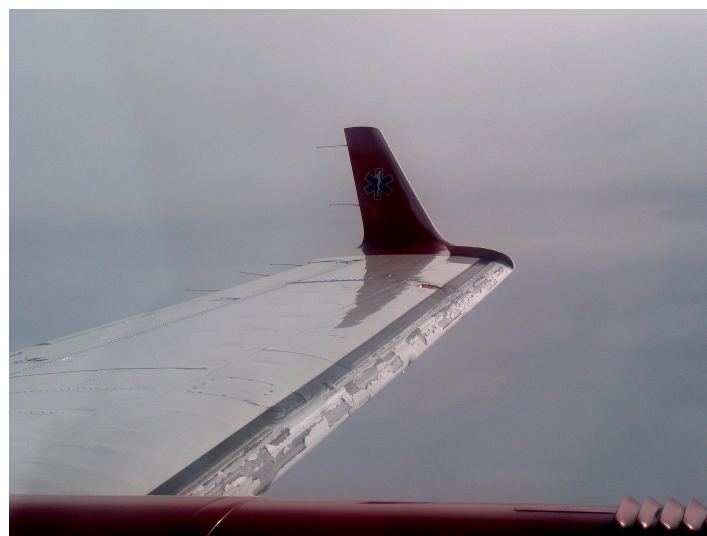
Figure 1. Ice accretion on the wing's leading edge [15].
