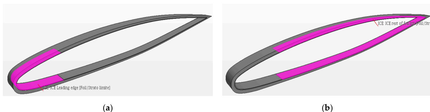
Figure 8. De-ice model setup: (a) Heated Part; (b) Non Heated Part.
