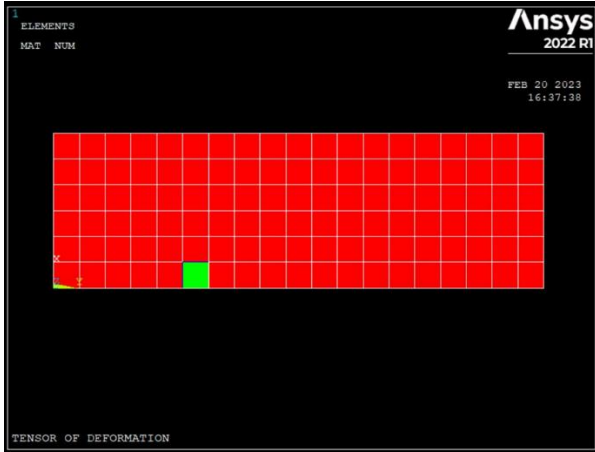
Figure 5: critical element (in green) of the lattice section from the static analysis on the homogenized lattice
