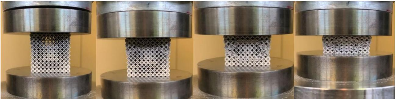
Figure 2: compression test of the  $bccz$  sample graded using process P1
