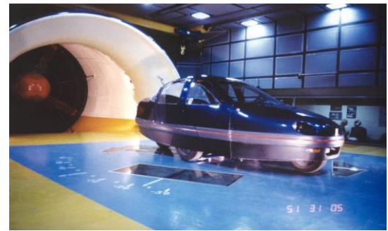
Figure 10. Rhomboid arrangement of the wheels: experimental chassis with central driving wheels and rear wheel without a braking device (above) and the “PRIMA” car (below) with front and rear steering wheels and with a central driving axle in the Pininfarina wind tunnel
