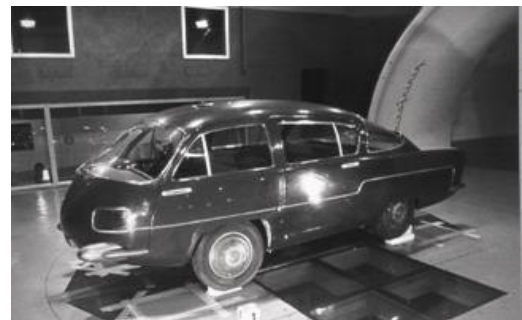
Figure 5. The M1000 model in the wind-tunnel at the Politecnico di Torino in 1953 (above) and a full-scale car in the Pininfarina wind-tunnel in 1977, where a C_x = 0.295 was found (below)
