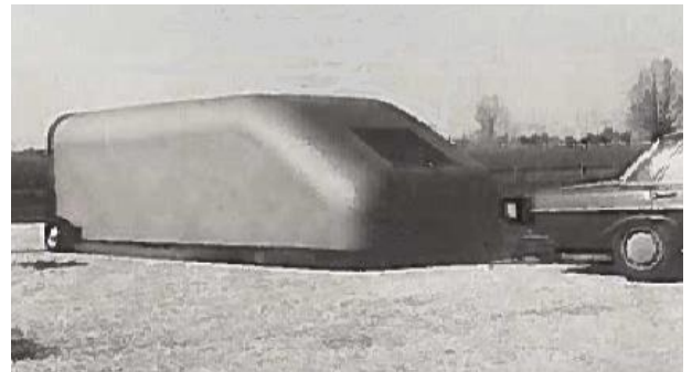
Figure 13. Trailer used to determine the rolling resistance of a vehicle [11]
