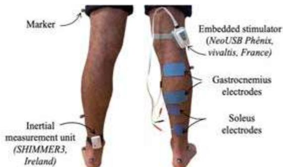
**Figure 1:** Experimental device
