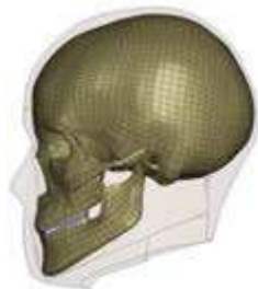
Figure 1: The skeletal mesh, with the surrounding soft tissues shown in transparent shading.
