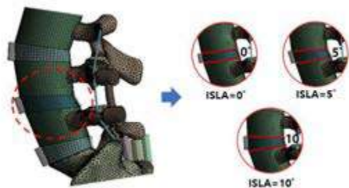
Figure 1: Finite element models of L3-S1 with different lordosis angle between PLIF segment.
