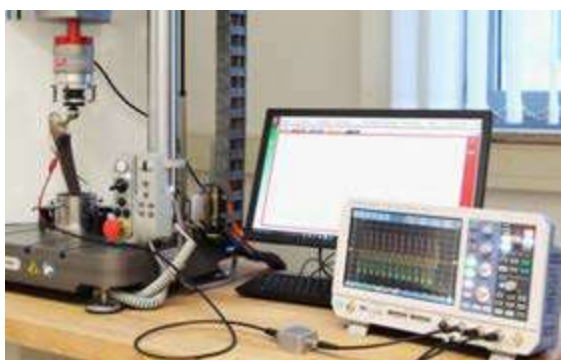
Figure 1: Experimental measurement setup-Application of different force profiles to the energy-autonomous hip implant.
