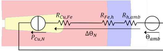
Fig. 8. Simplified thermal network for non-ventilated machines.
