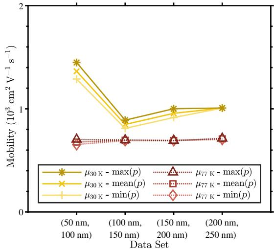
FIG. 7. The intrinsic vertical hole mobility calculated using the resistance scaling method for pairs of calculations with consecutive simulations sizes at temperatures of 30 K (yellow lines) and 77 K (red dotted lines). The mobility is calculated using three different values for the hole density: the maximum, the mean, and the minimum of the two calculations in the pair.
