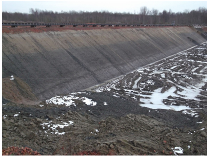
Figure 3. Clay layer at the overburden: the material is exploited for brick production (credits C. Oggeri).
