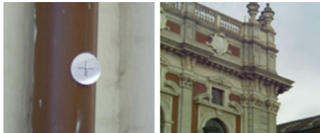
Figure 2: Example of a retroreflective target used during measurements (left) and natural point (right).
