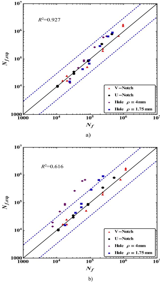
Fig. 4. Number of cycles to failure for different notched samples made of EN3B steel ( $R = -1$ ): experimental data [5] vs. FFM predictions according to the average a) and the pointwise b) formulations. The dashed lines represent 1/3 and 3 scatter bands.
