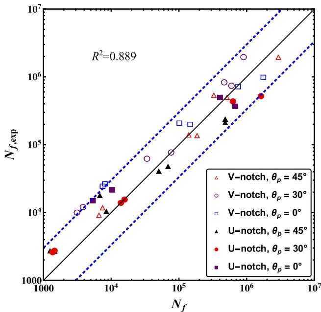
Fig. 9. Number of cycles to failure for different notch geometries and manufacturing angles, PLA ( $R = 0$ ): experimental data [13] vs. FFM predictions. The dashed lines represent 1/3 and 3 scatter bands.
