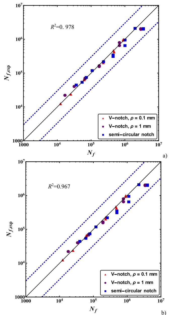
Fig. 10. Number of cycles to failure for different notched samples made of Inconel 718 ( $R = 0$ ) [58]: experimental data vs. a) FFM, b) TCD predictions. The dashed lines represent the scatter bands of 1/3 and 3.
