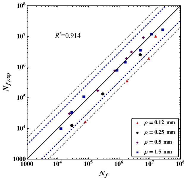
Fig. 7. Number of cycles to failure for samples weakened by a circular hole: experimental data on Al 2024-T351 ( $R = -1$ ) [49] vs. FFM predictions. The dashed blue lines represent the scatter bands of 1/3 and 3, whereas the dotted-dashed gray lines illustrate the scatter bands of 1/5 and 5. (For interpretation of the references to colour in this figure legend, the reader is referred to the web version of this article.)
