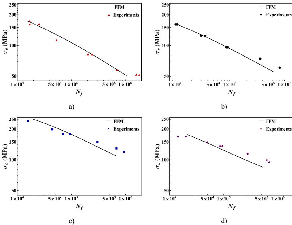
Fig. 3. Nominal (gross-section) stress amplitude vs. number of cycles to failure for different notched samples made of EN3B steel ( $R = -1$ ), a) V-notch, b) U-notch, c) Hole  $\rho = 1.75$  mm, d) Hole  $\rho = 4$  mm. Solid black lines refer to the predictions by average FFM formulation (Eq. (7)) and the experimental data from [5] are shown by markers.
