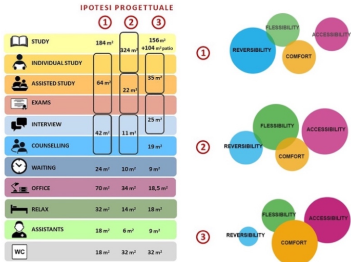
Figure 3. Comparison between the three design hypotheses and evaluation according to the established project requirements: flexibility, reversibility, comfort, accessibility.
