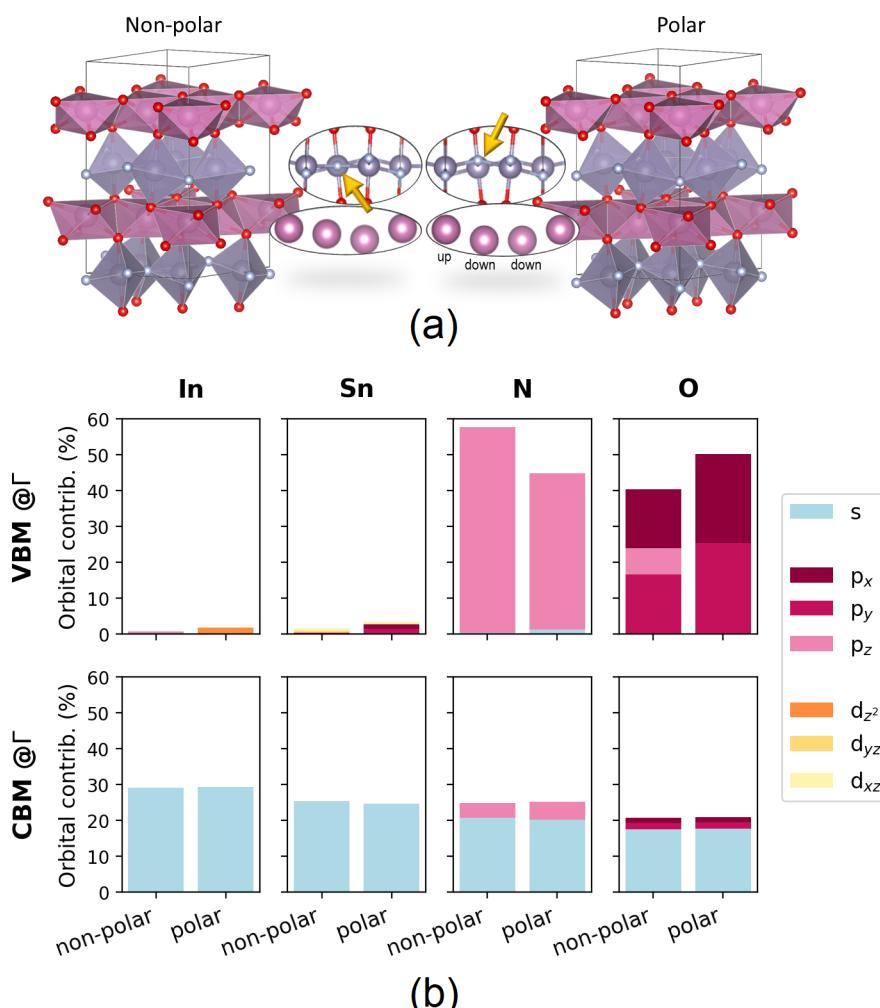
**Figure 1.** (a) Left, optimized nonpolar and, right, polar structures of  $\text{InSnO}_2\text{N}$ . For both systems in the inset, the alignment of Sn atoms is reported [large gray, Sn; small silver, N; large purple, In; small red, O atoms]; (b) orbital contribution (%) to the band edges (VBM/CBM) at  $\Gamma$  point for the two, nonpolar and polar, systems.
