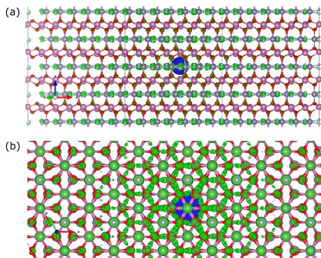
**Figure 5.** (a) Lateral and (b) top view of the first bright exciton in the nonpolar structure. The green isosurface ( $1.75 \times 10^{-7} \text{ e}/\text{\AA}^3$ ) is the electronic (de)localization associated with the hole position (blue large sphere) [large gray, Sn; small whiteish, N; large purple, In; small red, O atoms].
