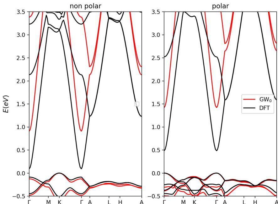
**Figure 2.** Electronic bandgap calculated for the nonpolar (left) and polar (right) structures of  $\text{InSnO}_2\text{N}$ . ( $\Gamma = 0, 0, 0$ ;  $K = -0.333, 0.667, 0.0$ ;  $M = 0.0, 0.5, 0.0$ ;  $A = 0.0, 0.0, 0.5$ ;  $L = 0.0, 0.5, 0.5$ ;  $H = -0.333, 0.667, 0.5$ ) [black, PBE; red,  $e\text{-}GW$ ].
