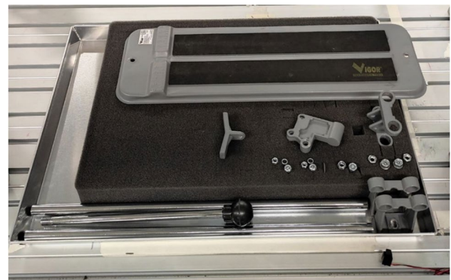
Fig. 3 Tray with workpieces of the tile cutter
