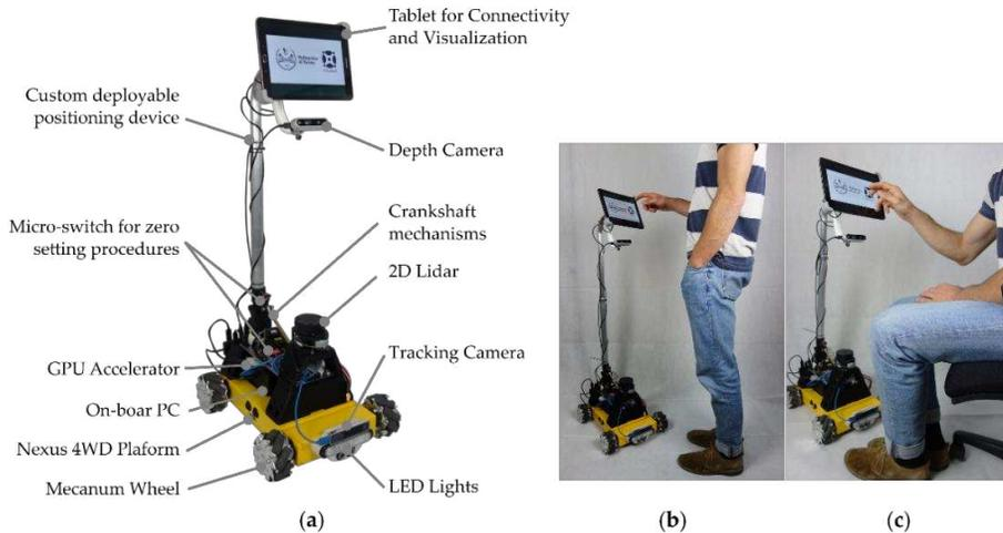
Fig. 2 Marvin prototype: (a) main components of the assistive robot, (b) deployed configuration for better-standing usage, tablet height = 1.1 m, tilting mechanism angle =  $0^\circ$ , (c) retracted and angled configuration for better-seated usage, tablet height = 0.80
