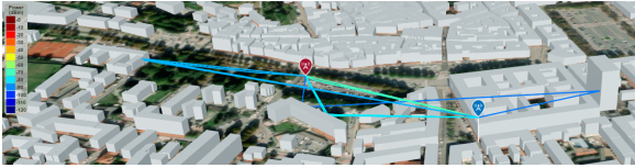
Fig. 4: Ray tracing with multiple propagation paths between the transmitter and the receiver.
