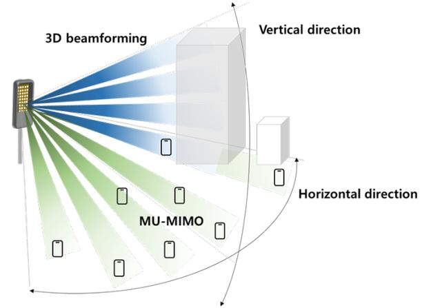
Fig. 2: Illustration of the concept of Massive MIMO.
