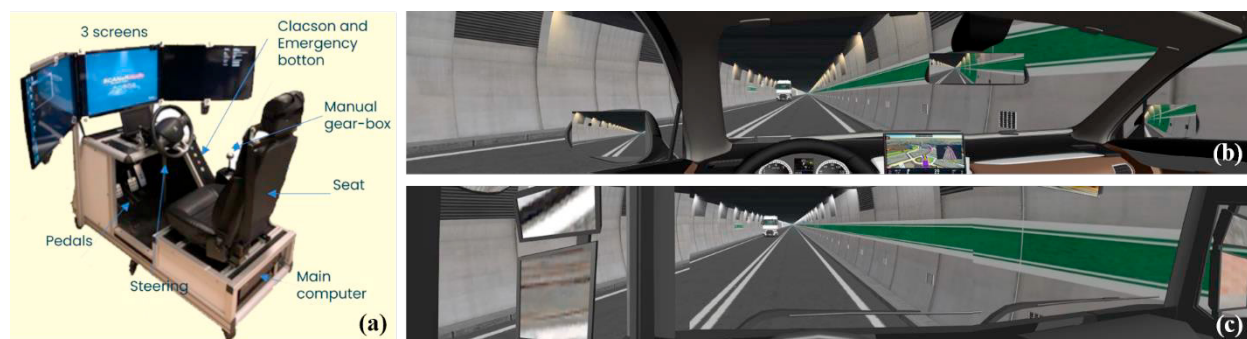
Fig. 1. (a) Fixed-base driving simulator (Road Safety and Driving Simulation Laboratory, Politecnico di Torino); (b) Simulated car cockpit and engine in the virtual environment; (c) Simulated truck cockpit and engine in the virtual environment.
