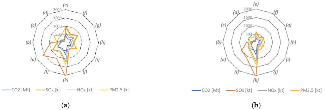
Figure 3. (a) Emissions of pure HVAC grid. (b) Emissions of hybrid HVAC-HVDC grid.
