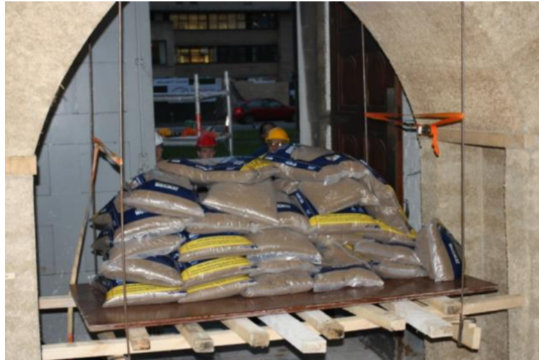
Figure 3: Structural testing of the hemp lime vault
