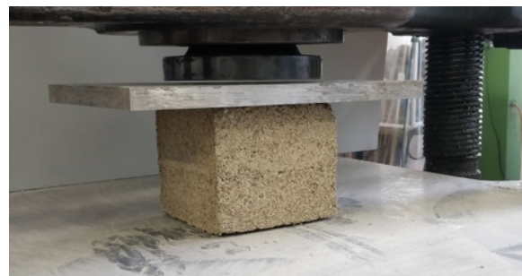
Figure 12: Compression tests of brick and cube samples
