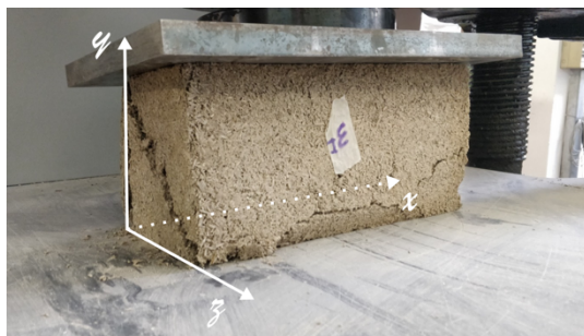
Figure 12: Compression tests of brick and cube samples
