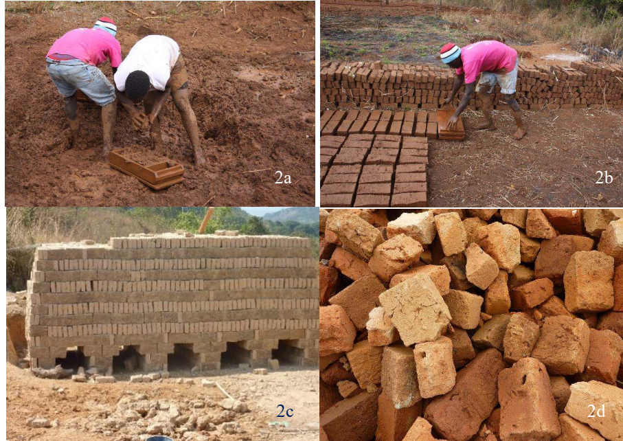
Fig. 2. Production techniques of fired clay bricks in Tanzania
