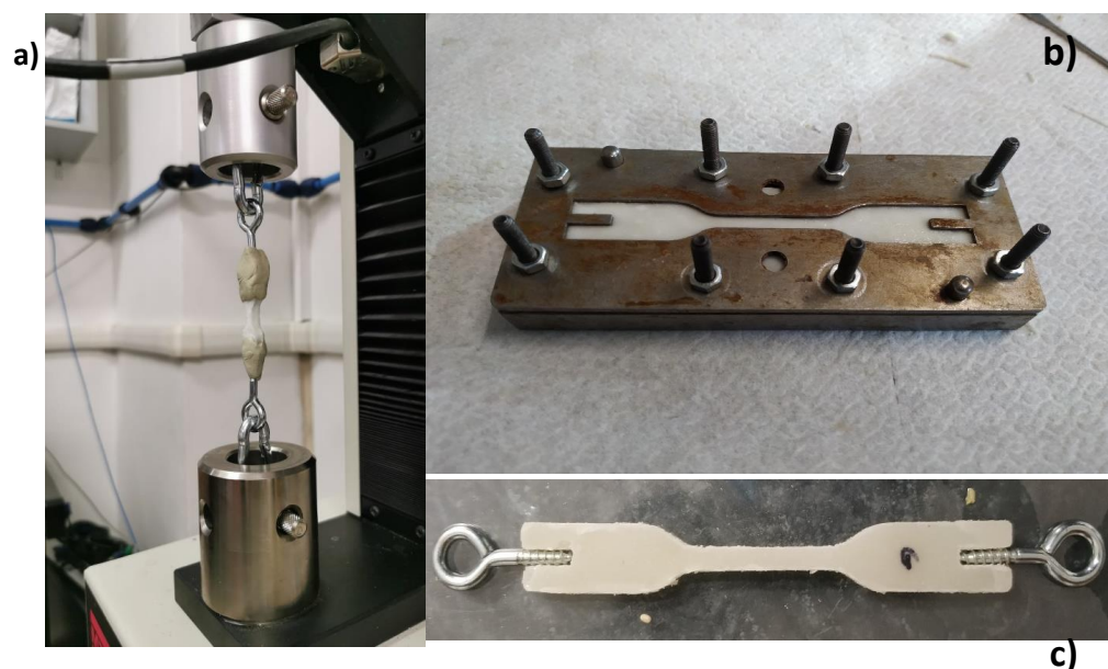
Figure 6. (a) Tensile test set-up; (b) baseplate and plates stacked during samples preparation; (c) multi-layer sample with eyelets.
