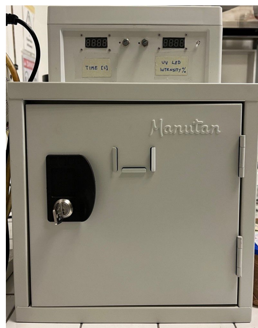
Figure 4. UV-curing prototype box.
