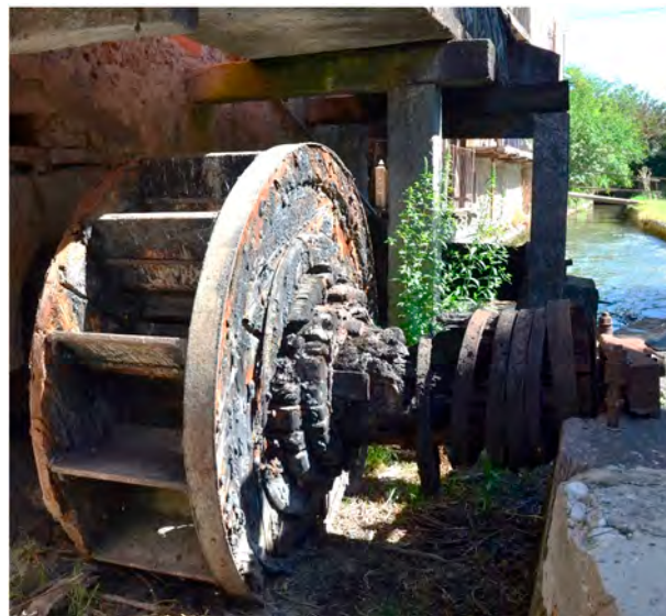
Figure 17. Water wheel #2 powering tilt hammer #2.
