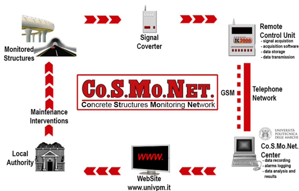
Figure 2. The Co.S.Mo.Net monitoring system.
