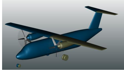
Fig. 10 Aircraft baseline as results of the MDA.
