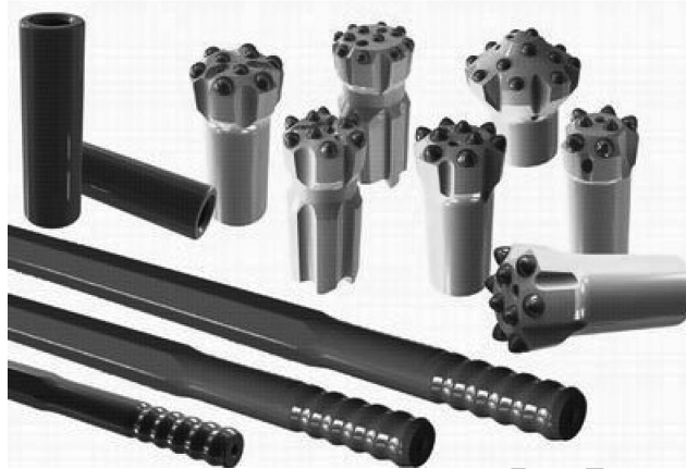
Figure 2.8 A wide selection of bits is available. To achieve optimum life and grinding interval as well as penetration rate, bit design, carbide grade and button shape must be selected depending on rock conditions.
