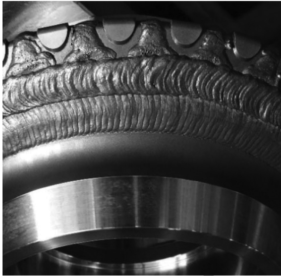
Figure 2.36 Special disk cutter with tungsten carbide inserts for extremely abrasive and hard rocks.
