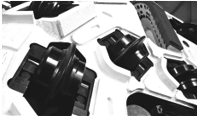
Figure 2.30 Detail of the front plate and wear protection.
