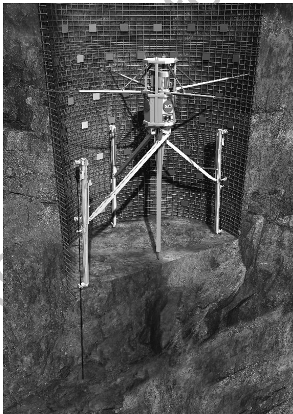
Figure 2.129 Example of shaft drilling jumbo. (Courtesy of Herrenknecht.)
