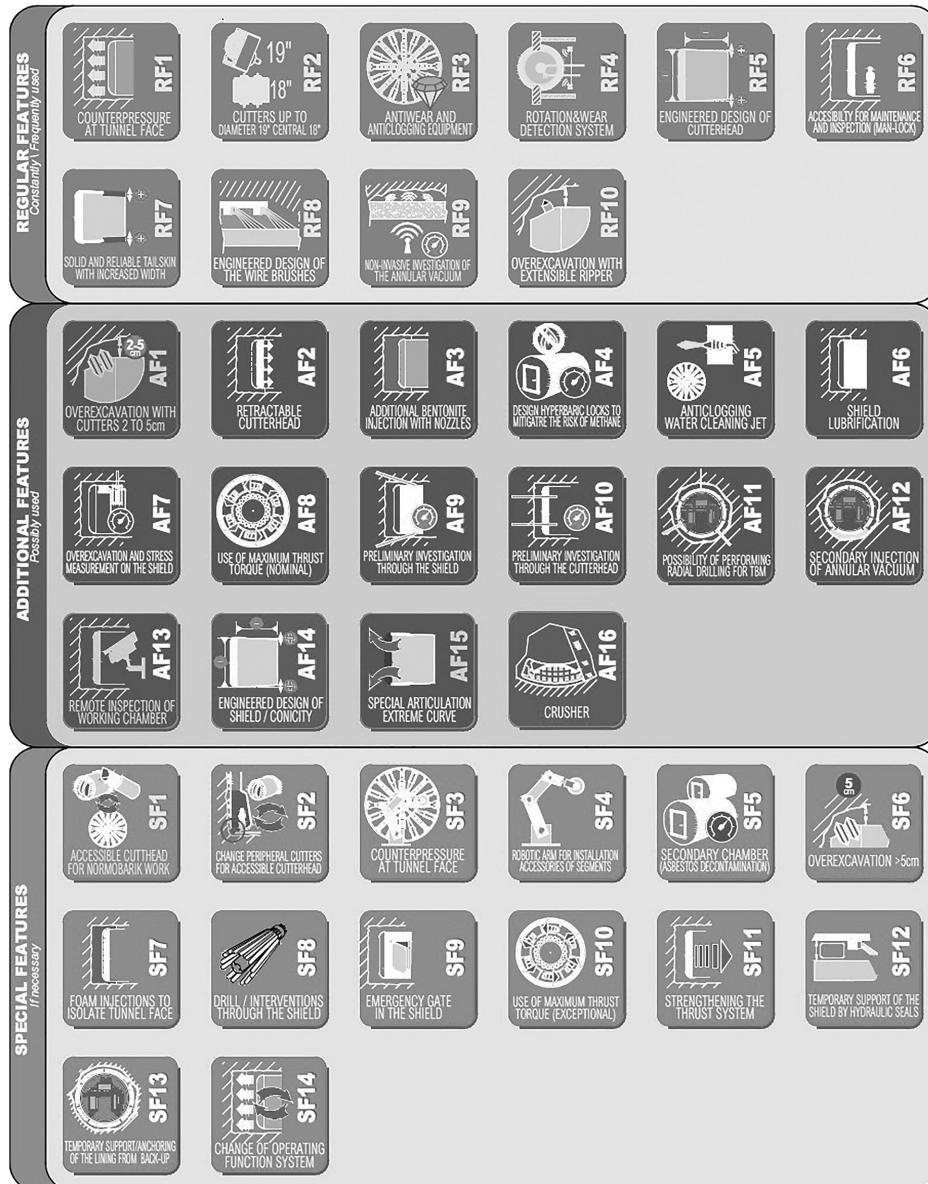
Figure 2.112 Regular, additional and special features for actual Earth Pressure Balance TBMs. (Courtesy of Geodata.)
