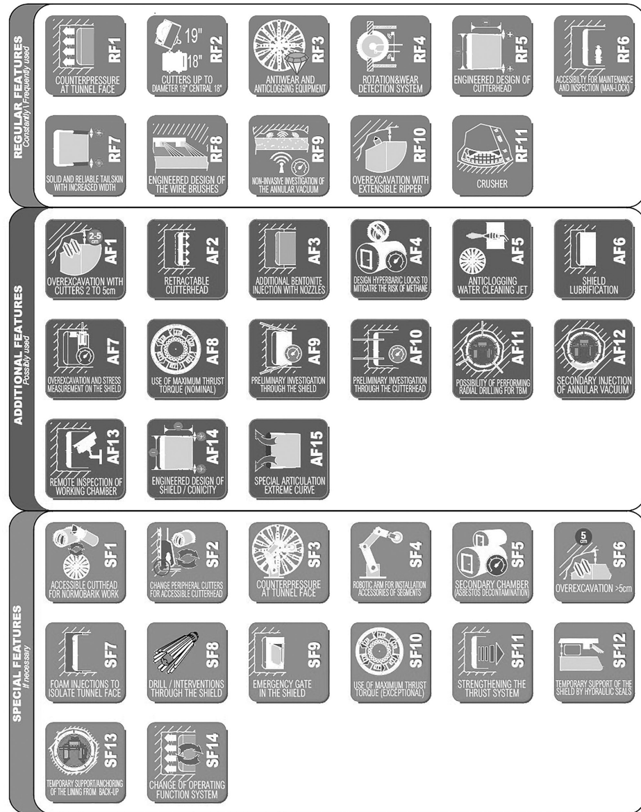
Figure 2.113 Regular, additional and special features for actual slurry type machines.
