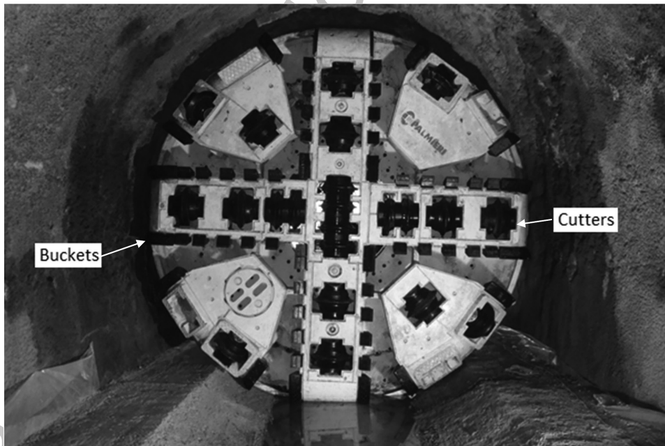
Figure 2.31 Front loading type cutterhead adopted for the excavation of a tunnel in variable conditions through soft Siltstone and hard and abrasive gneiss in Algeria.
