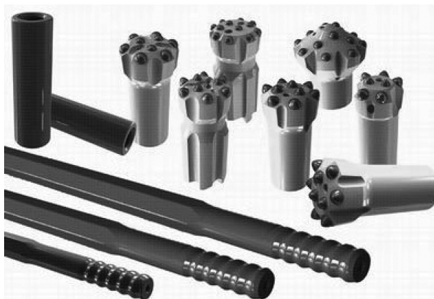
Figure 2.8 A wide selection of bits is available. To achieve optimum life and grinding interval as well as penetration rate, bit design, carbide grade and button shape must be selected depending on rock conditions.
