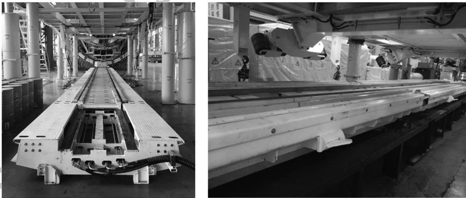
Figure 2.46 Photograph of the segment feeder.
