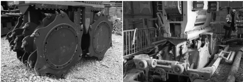
Figure 2.144 Trench cutter excavation and wall construction process - guide frame and cutter wheels. (Courtesy of Liebherr.)
