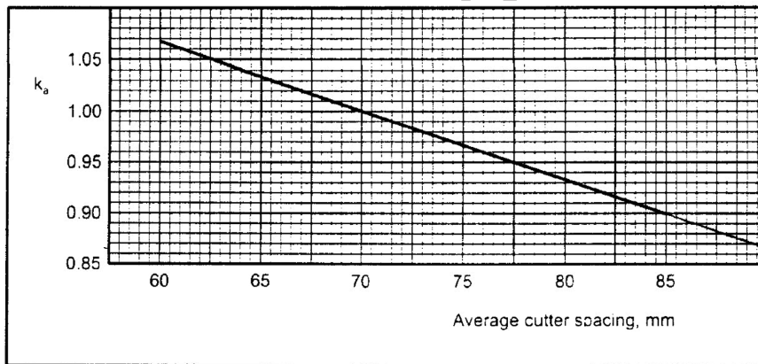
Figure 2.78 Diagram for k_a assessment (Bruland, 1998).
