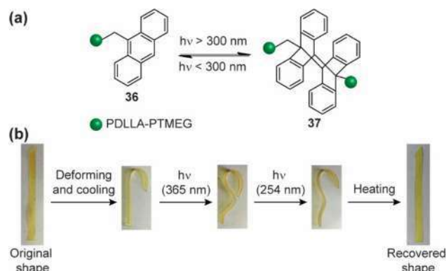
Figure 12. (a) Schematic representation of the photo cross-linking of 36. (b) Reprinted with permission from ref 130. Copyright Elsevier.
