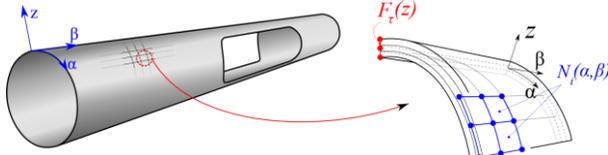
Fig. 1. Representative tape-spring hinge and advanced shell model
