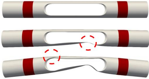
Fig. 5. Deformed configuration at 0°, 2° and 12° respectively.
