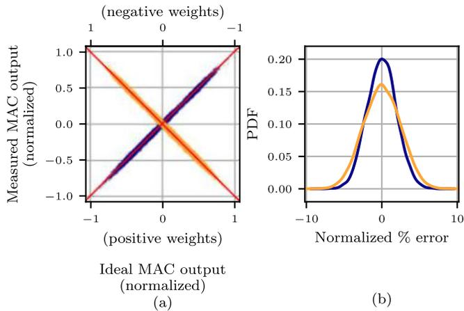
Fig. 2. Accuracy of the AIMC unit: (a) Measured MAC operations as a function of the ideal MACs, where MAC coefficients are implemented with programmable integrated resistances. MAC weights  $w_i$  employed for the yellow (purple) data are negative (positive). (b) MAC error distributions of the two data sets.
