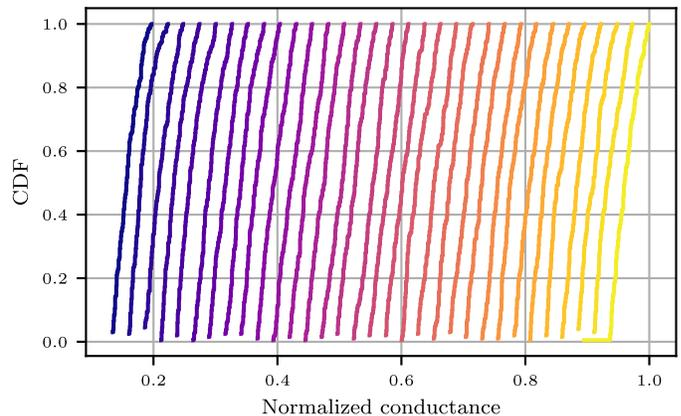
Fig. 4. CDFs of 32 levels of programmed cell conductances.
