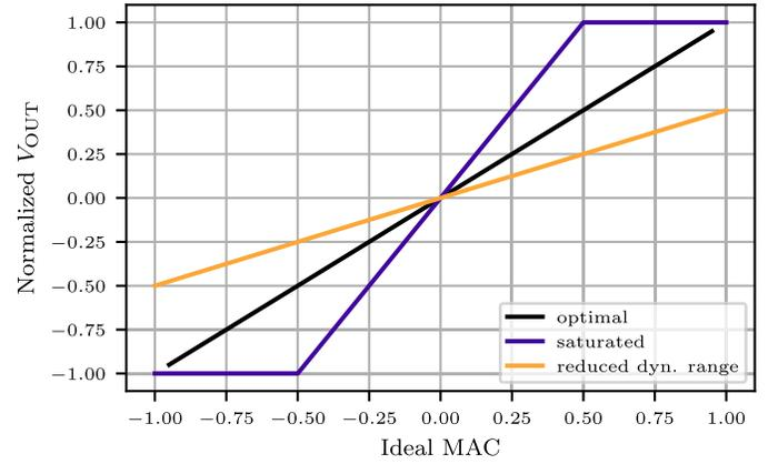
Fig. 5. Effects of different values for the reference conductance  $g_{\text{REF}}$  on the output swing of the MACs. *i*) optimal swing (Equation (6)); *ii*) saturation due to low  $g_{\text{REF}}$  level; *iii*) swing reduction induced by PCM cells drift with constant  $g_{\text{REF}}$ .
