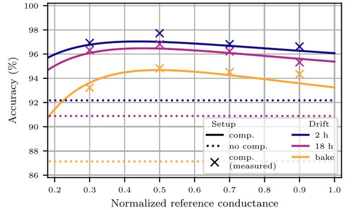
Fig. 6. MAC accuracy as a function of  $\frac{g_{\text{REF}}}{g^{\text{MAX}}}$ . Continuous lines refer to simulated results after 2- and 18-hours room temperature and 90°C bake drift. Dashed lines represent the MAC accuracy in the same conditions when no compensation is adopted. Crosses report the results of experimental evaluation of MAC accuracy for different  $g_{\text{REF}}$  levels.
