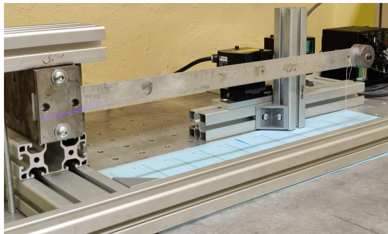
Figure 1. Euler–Bernoulli cantilever beam.
