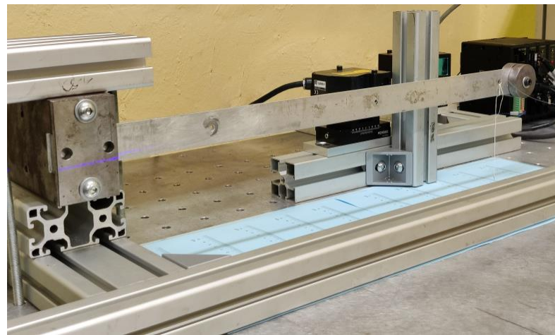
Figure 1. Euler–Bernoulli cantilever beam.
