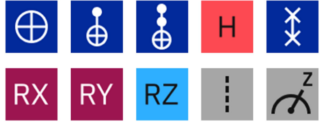
Fig. 1. Icons showing the quantum gates and the operations described as shown in the IBM Quantum Composer [39], [40]. From left to right, top to bottom: NOT gate, CNOT gate, Toffoli gate, Hadamard gate, SWAP gate, RX gate, RY gate, RZ gate, barrier operation, and measurement operation.
