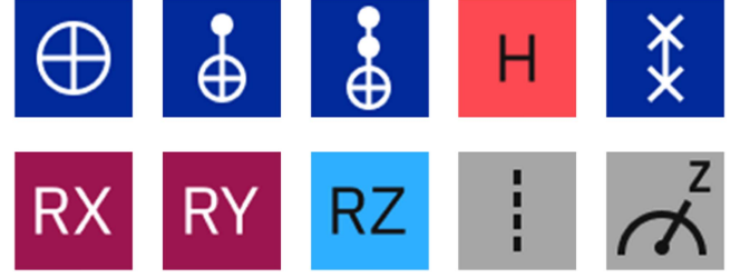
Fig. 1. Icons showing the quantum gates and the operations described as shown in the IBM Quantum Composer [39], [40]. From left to right, top to bottom: NOT gate, CNOT gate, Toffoli gate, Hadamard gate, SWAP gate, RX gate, RY gate, RZ gate, barrier operation, and measurement operation.
