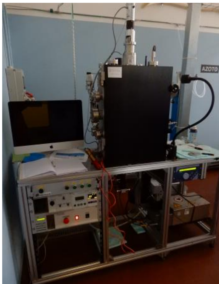
Figure 14: Homebuilt RF sputtering system used for the gold deposition in the QR Laboratories at INRiM.
