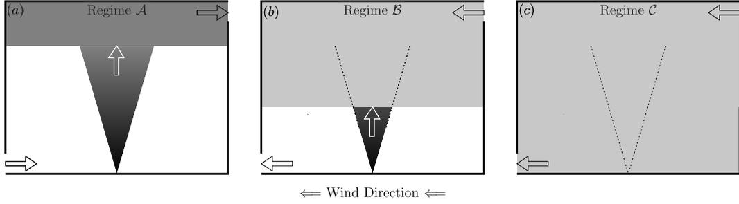
Figure 2: The three possible regimes that form when the top opening is in the upwind wall and wind contrasts the buoyancy-induced natural ventilation: regime  $\mathcal{A}$ , “stratified forward flow” (a); regime  $\mathcal{B}$ , “stratified reverse flow” (b); regime  $\mathcal{C}$ , “mixed reverse flow” (c). Wind direction is from right to left.
