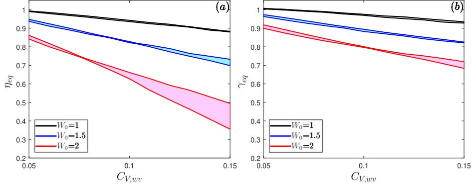
Figure 6: Effect of the noise parameters  $C_{V,ww}$  on the average interface elevation  $\eta_{eq}$  (a) and average reduced gravity  $\gamma_{eq}$  (b). The dimensionless correlation time  $\hat{\tau}_{wv}$  was varied from 0.05 (highest curves for a given  $W$ ) to 0.15 (lower curve). Shaded areas refer to values of  $\hat{\tau}_{wv}$  between these two boundaries. The venting parameter is  $V = 1$ .
