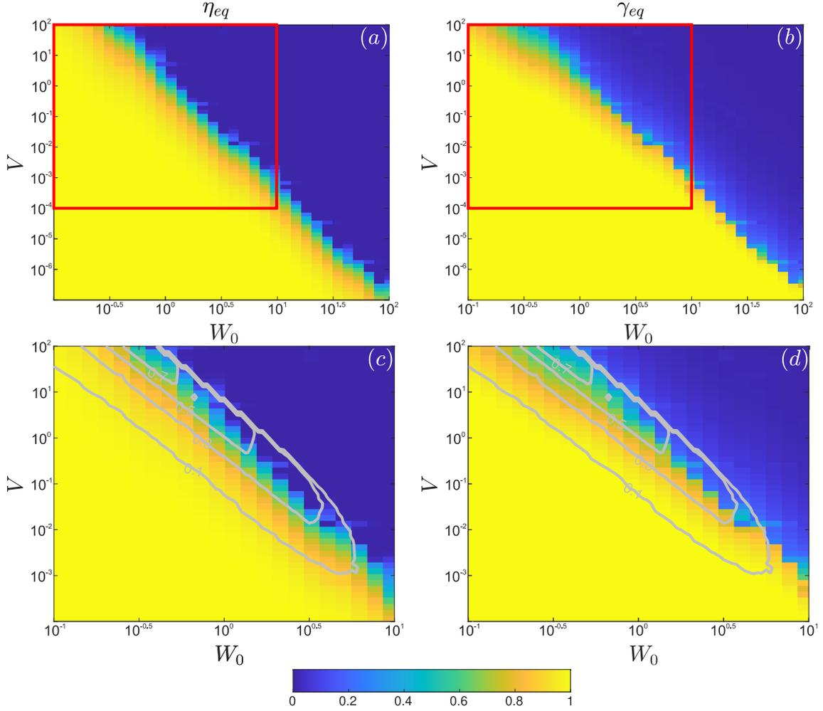
Figure 7: Effect of the venting parameter  $V$  and mean wind  $W_0$  on  $\eta_{eq}$  (a) and  $\gamma_{eq}$  (b). The figure reports the largest attained deviations of  $\eta_{eq}$  and  $\gamma_{eq}$  from unity.  $C_{V,ww}$  and  $\hat{\tau}_{wv}$  spanned ranges  $[0.05-0.15]$  and  $[0.01-0.1]$ , respectively. Red rectangles delimit the zoomed view reported in panels (c) and (d). The gray curves are iso-lines of the “overshoot” ( $\hat{h}_0 - \hat{h}_{\min}$ ) as defined in [17].
