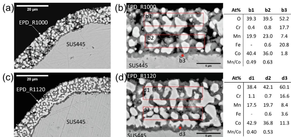
**Fig. 3.** FE-SEM cross-section images (backscattered electrons) at different magnifications of coatings after reduction treatment, with EDX elemental analysis of regions and points marked in the red colour of EPD\_R1000 (a,b) and EPD\_R1120 (c,d) samples.
