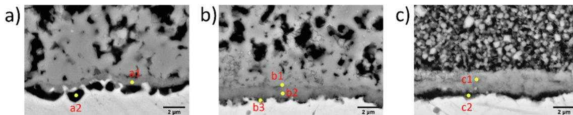
Fig. 8. FE-SEM cross sections images (backscattered electrons) of steel substrate/EPD coatings interface after ASR test: EPD\_R1000 (a), EPD\_R1120 (b), EPD\_Ox (c). EDX elemental analysis of points marked in the yellow colour is reported in Table 3.
