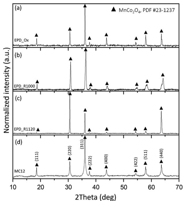
**Fig. 4.** XRD patterns of EPD\_Ox coating (a), EPD\_R1000 coating after reoxidation (b), EPD\_R1120 coating after reoxidation (c) and MC12 powders (d) indexed in cubic unit cells according to  $\text{MnCo}_2\text{O}_4$  phase as included in the PDF Database.
