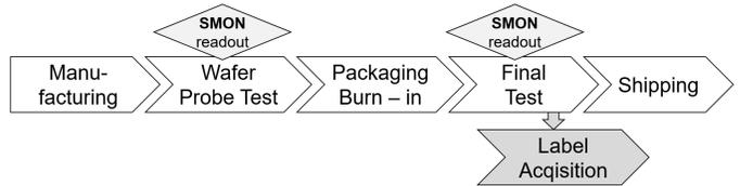
Fig. 1. Data collection steps through the manufacturing
