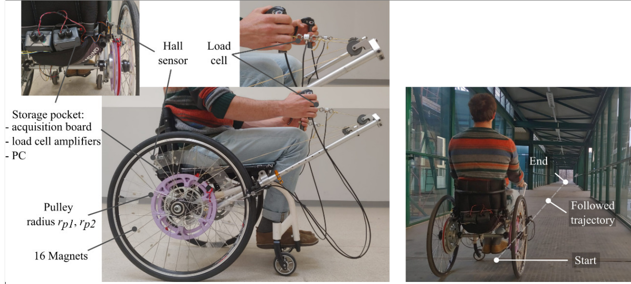
Fig. 4. Handwheelchair.Q experimental setup.
