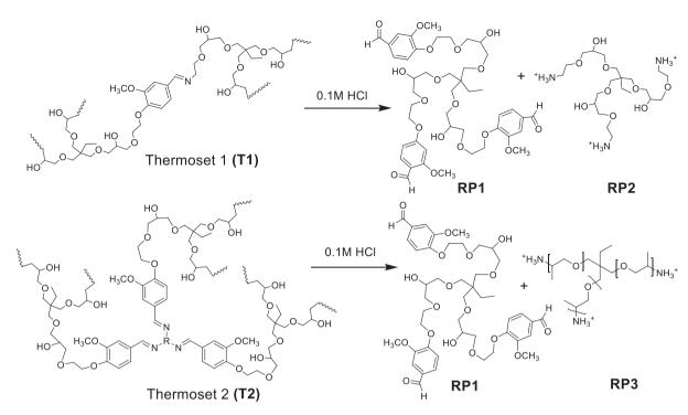
Figure 8. Suggested schematic diagram for the chemical recycling pathway of thermoset 1 (T1) and 2 (T2) to different recycled products (RP1, RP2, and RP3).
