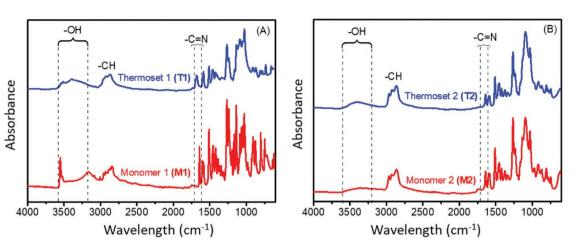
Figure 4. FT-IR spectra of A) monomer 1 (M1) and corresponding thermoset 1 (T1), B) monomer 2 (M2) and corresponding thermoset 2 (T2).
