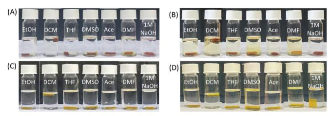
Figure 5. A,C) Initial and B,D) final images of thermoset 1 (TI) and 2 (T2) after subjection to different solvents at room temperature for 48 h.
