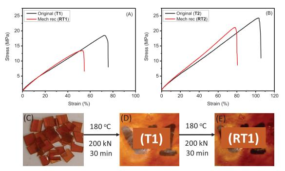
Figure 9. Representative stress-strain curves of A) thermoset 1 (T1) and B) thermoset 2 (T2) after first compression molding and after mechanical recycling by second compression molding cycle (RTI and RT2). Digital photos of thermoset 1 (TI): C) Cut pieces of oven cured thermosets, D) compression molded original thermoset (T1), and E) recycled, second time compression molded thermoset (RT1).
