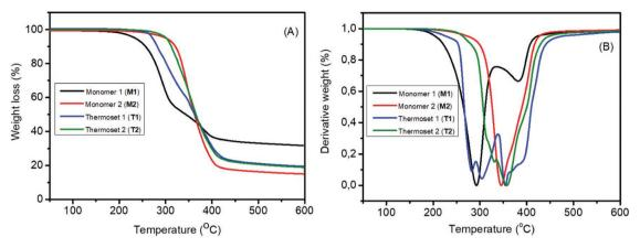
Figure 6. TGA analysis showing the A) weight loss and B) first derivative weight loss curves of monomer 1 (M1) and 2 (M2) as well as thermoset 1 (T1) and 2 (T2).
