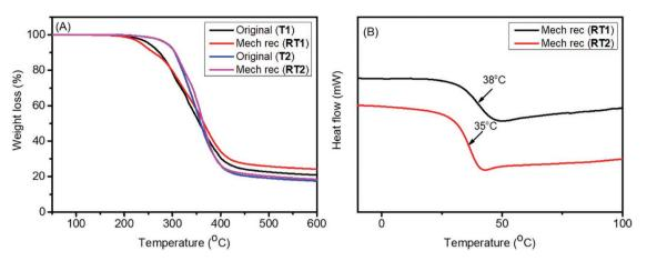
Figure 10. A) TGA and B) DSC curves mechanically reprocessed thermosets 1 (RTI) and thermoset 2 (RT2).
