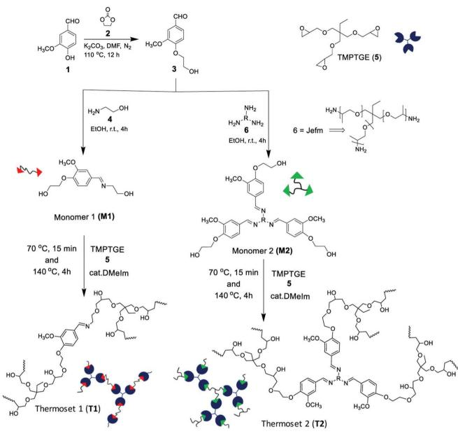
Figure 3. Schematic illustration of the synthesis of Schiff-base based thermosets 1 (T1) and 2 (T2).
