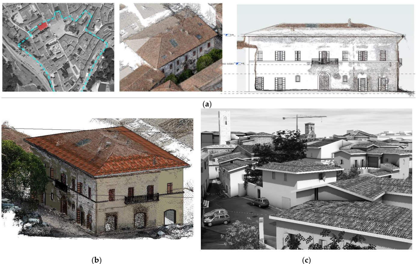
Figure 8. Examples of of one sample building definition (building n°2, Via Solferino) based on point clouds with parametric modeling, with eaves, ridges, floors and ground lines (a); corresponding modelling according to LOD 300 (b) in the evacuated residential area; and aerial views of the centre with the other modeled buildings (c).
