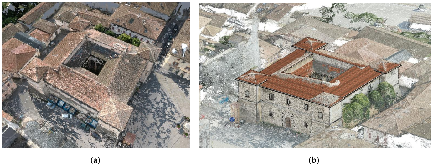
Figure 11. Examples of volumetric high scale 3D data: point cloud (a), and (b) models for Castellina building in Norcia.
