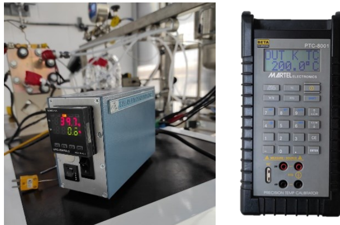
Figure 2.21 left: Temperature controller – right: Instrument used for the thermocouple calibration
