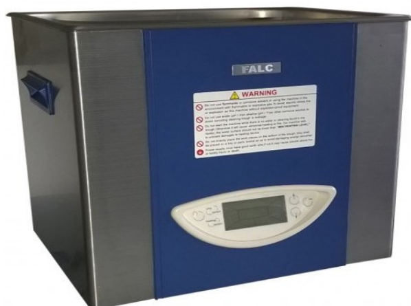
Figure 2.14 Ultrasonic Cleaner used in cell preparation.
