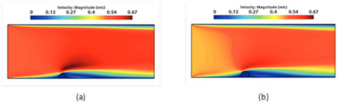
**Figure 5.** Velocity contour profile over a kernel extrapolated from the CFD simulation. With an airstream profile of 0.5 m/s note, the higher speed (dark red) over the point of the kernel of spinoso maize (a) compared to the control variety (b). This higher speed increases the turbulence intensity downstream enhancing the drying process.
