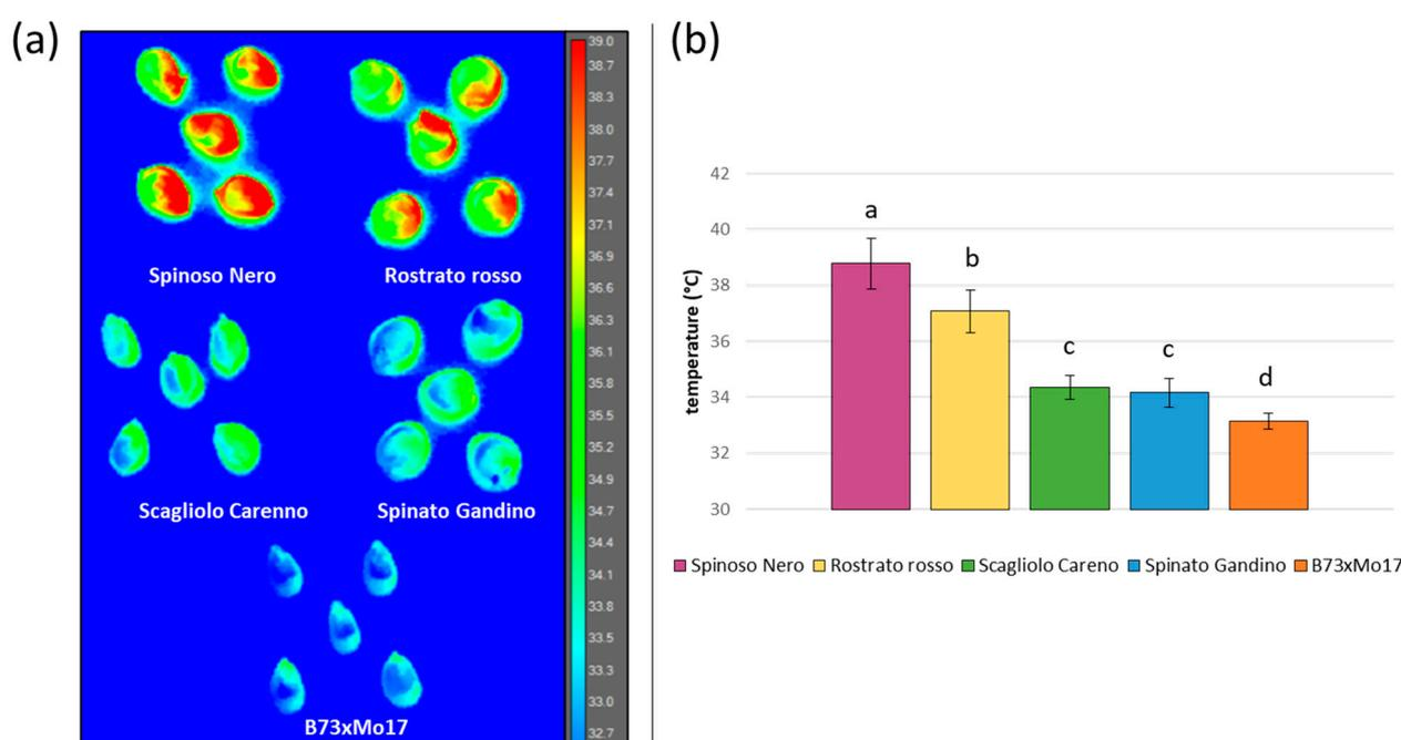
**Figure 9.** (a) Representative image of the seed temperature acquired with the thermographic camera (FLIR T650sc). (b) Seed temperature of the Italian traditional varieties and B73/Mo17 (control). Statistical analysis was performed using ANOVA test ( $p < 0.05$ ) and Tukey test.
