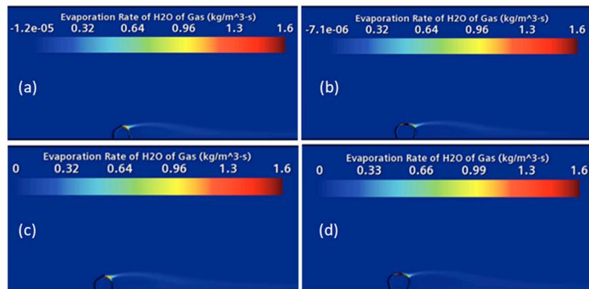
**Figure 6.** Evaporation Rate  $\left[ \frac{Kg}{m^3 \cdot s} \right]$  at different timings extrapolated from the CFD simulation. (a) Nero Spinoso at 0.5 s; (b) control (B73/Mo17 hybrid) at 0.5 s; (c) Nero Spinoso at 1 s; (d) control at 1 s.
