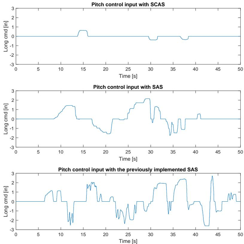
**Fig. 13 The longitudinal control input provided by the pilot during a take-off in helicopter mode followed by a conversion to airplane mode. The longitudinal control input is analyzed considering a flight with the SCAS active, a flight with only the SAS, and with the SAS originally implemented in [15]**
