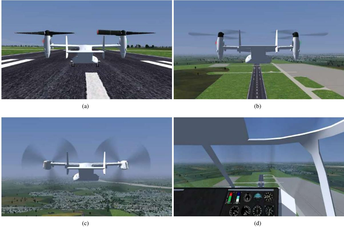
**Fig. 9** Screens captured from the FlightGear simulator. In (a), the aircraft on the ground is visualized from an external point of view. In (b), the tilt-rotor operates in helicopter mode with the position of nacelles at  $90^\circ$ . In (c), the tilt-rotor operates in airplane mode. In (d), the internal view of the aircraft with a Primary Flight Display consisting of several instruments
