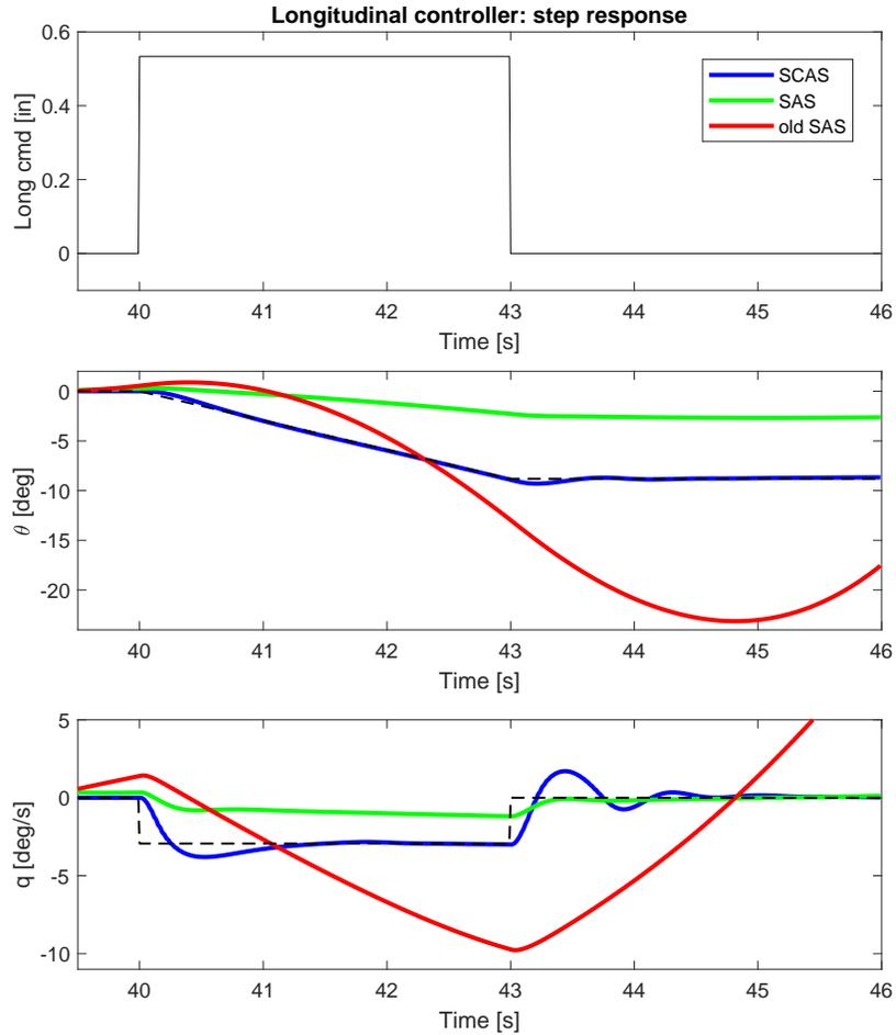
**Fig. 10** Aircraft response after a longitudinal input step. In blue the response with the SCAS active. In green is the response with only the SAS. In red is the response of the SAS originally implemented in [15]
