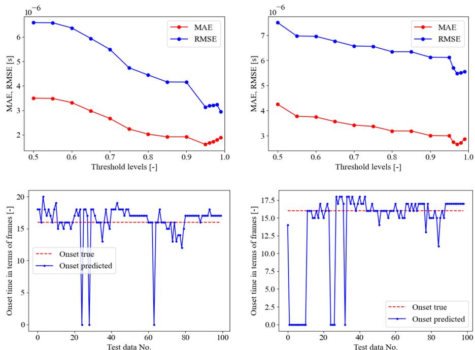
**Figure 11.** Fine-tuned SED on PLB test A. Upper pane, crack class probability threshold evaluation, lower pane onset time predictions in terms of frames on the PLB test sets B and C for optimal threshold. From left to right, PLB test B (optimal threshold of 99%), and C (optimal threshold of 98%). The onset time true values are always at a constant pre-trigger time of 256  $\mu$ s (frame No. 16).
