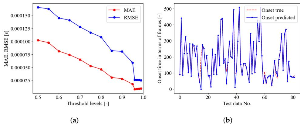
**Figure 6.** SED trained on seismic data only. (a) Crack class probability threshold evaluation in terms of MAE and RMSE; (b) onset time predictions in terms of frames on the test set (82 seismic data) for optimal threshold equal to 96%.
