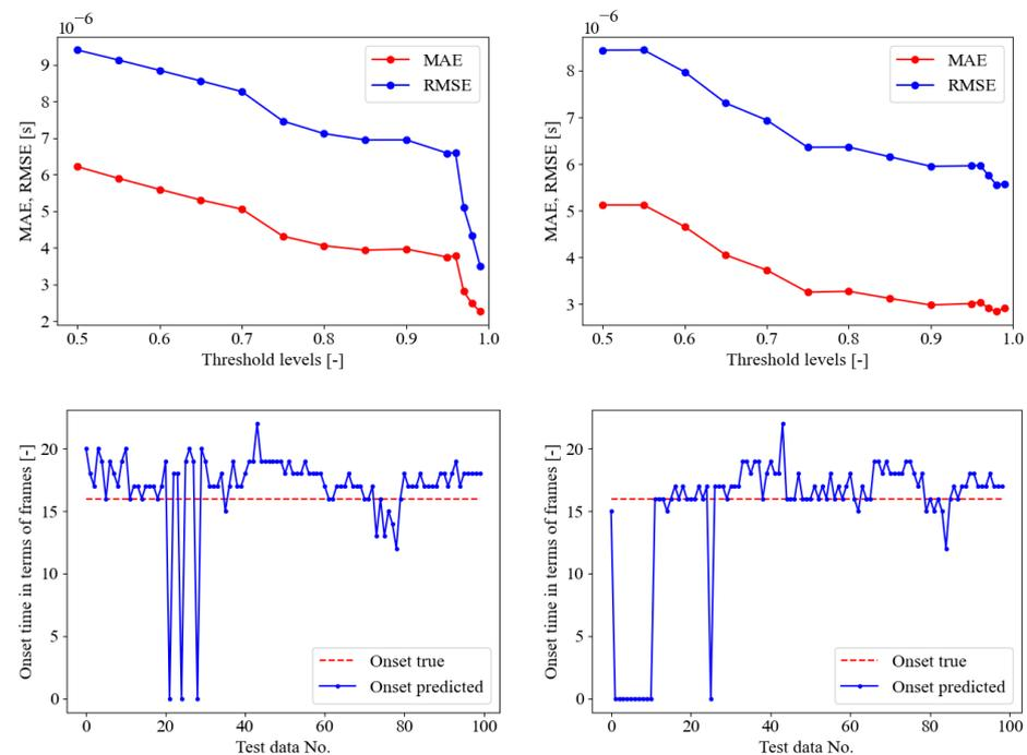
**Figure 9.** SED trained on AE only (training set: PLB test A). Upper pane, crack class probability threshold evaluation, lower pane onset time predictions in terms of frames on the PLB test sets B and C for optimal threshold. From left to right, PLB test B (optimal threshold of 99%), and C (optimal threshold of 98%). The onset time true values are always at a constant pre-trigger time of 256  $\mu$ s (frame No. 16).
