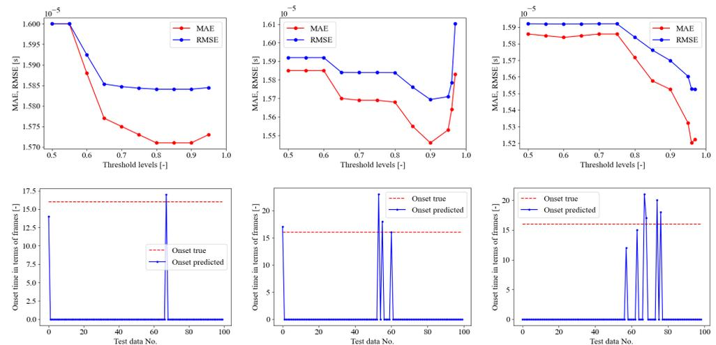
**Figure 7.** SED trained on seismic data only. Upper pane, crack class probability threshold evaluation, lower pane onset time predictions in terms of frames on the test set (82 seismic data) for optimal threshold. From left to right, PLB test A (optimal threshold of 85%), B (optimal threshold of 90%), and C (optimal threshold of 96%).
