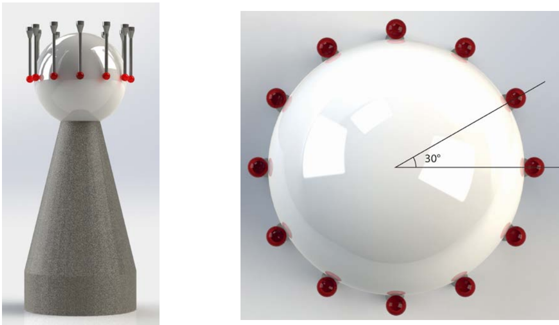
Figure 6: A “datum sphere” (with a diameter of 30 mm) was sampled in 12 different positions, with an angular spacing of 30°
