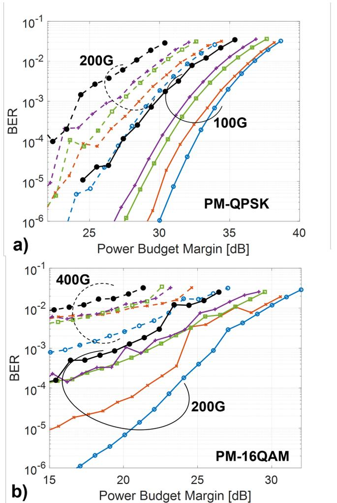
Fig. 5. Measured BER vs power budget margin for a) PM-QPSK and b) PM-16QAM modulation in different conditions: back-to-back (blue, circles), in 'OM3 only' (red, crosses), '3  $\mu\text{m}$  offset-OM3' (green, squares), '6  $\mu\text{m}$  offset-OM3' (purple, plus signs) and '3  $\mu\text{m}$  offset-OM3-3  $\mu\text{m}$  offset' (black, dots) configurations.
