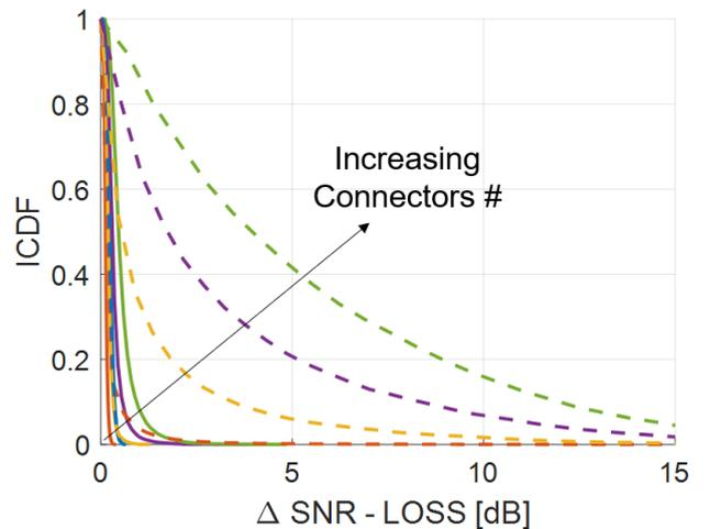
Fig. 3. ICDF of the  $\Delta SNR - Loss$  parameter in a  $25 \text{ GBaud}$   $220 \text{ m}$  OM3-based Coh-MMF system for number of connectors from 0 to 4 and for offset Rayleigh distribution mean of  $1 \mu\text{m}$  (solid) and  $3 \mu\text{m}$  (dashed).
