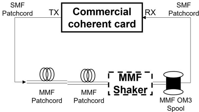
Fig. 4. Experimental setup of the Coh-MMF system.
