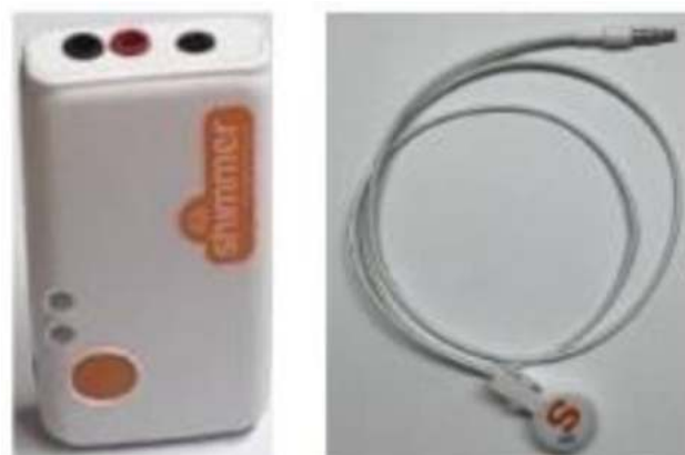
Figure 6. SHIMMER3 GSR+ Unit SR48-3-0 and SHIMMER PPG optical pulse clip for PPG recordings.
