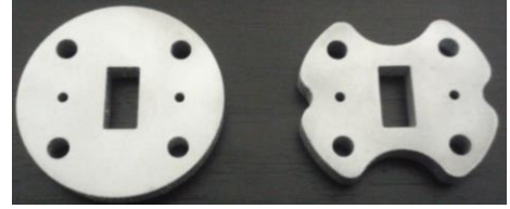
Fig. 8 Two of the nine prototypes of the WR51 waveguide lines manufactured in AlSi10Mg alloy to optimize the AM process parameter.
