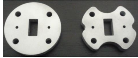
Fig. 8 Two of the nine prototypes of the WR51 waveguide lines manufactured in AlSi10Mg alloy to optimize the AM process parameter.
