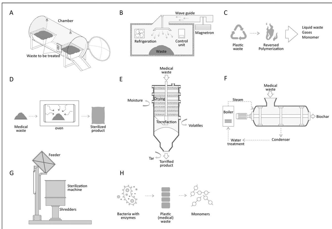
**Fig. 4.** Diagrams and schemes of low and medium thermal technologies. (A) Autoclave. (B) Microwave oven. (C) Depolymerization. (D) Dry heat treatment. (E) Torrefaction treatment. (F) Hydrothermal carbonization [56] (G) Converter machine [20]. (H) Biological treatment.
