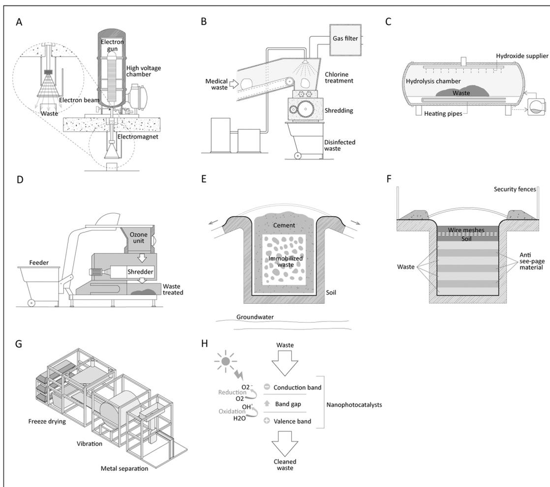
**Fig. 6.** Diagrams and schemes of physical-chemical technologies. (A) Electron beam (EB) treatment. (B) Chlorine disinfection treatment. (C) Alkaline treatment. (D) Ozonation process. (E) Immobilization treatment [105]. (F) Deep burial. (G) Promession process [109]. (H) Mechanism of nano photocatalysis.
